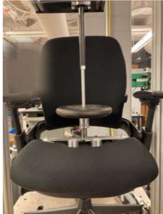
Figure 25. Steelcase Leap with the 25-mm LCI 300 seconds after nominal load was applied
