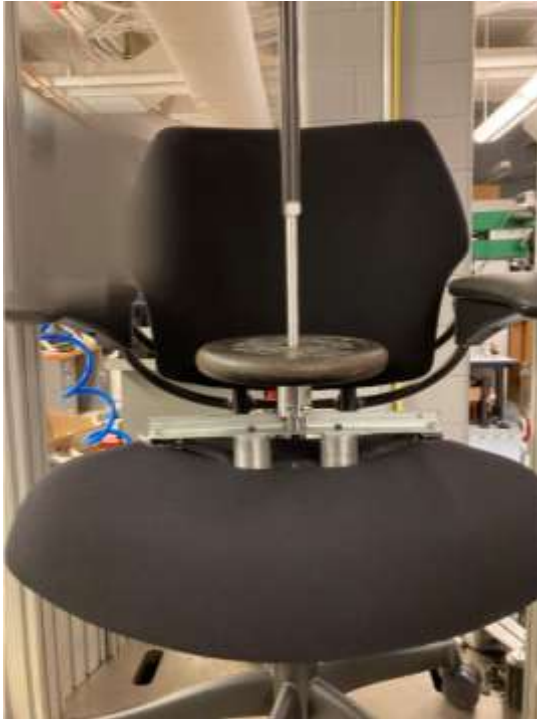
Figure 20. Humanscale Freedom with the 40-mm LCI 300 seconds after nominal load was applied
