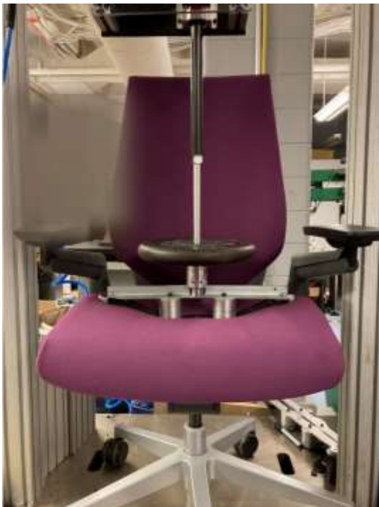
Figure 22. Steelcase Gesture with the 40-mm LCI 300 seconds after nominal load was applied
