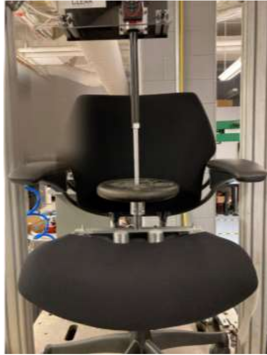
Figure 21. Humanscale Freedom with the 25-mm LCI 300 seconds after nominal load was applied
