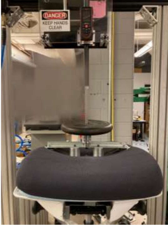
Figure 16. Anthros Chair with the 40-mm LCI 300 seconds after nominal load was applied
