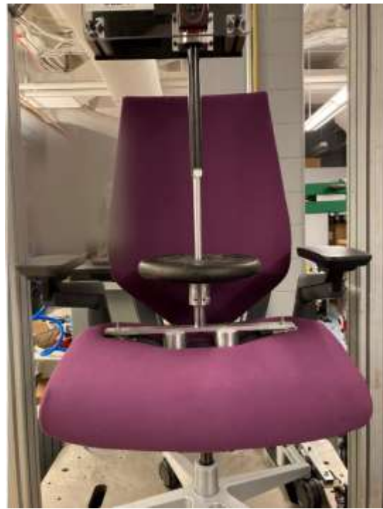
Figure 23. Steelcase Gesture with the 25-mm LCI 300 seconds after nominal load was applied
