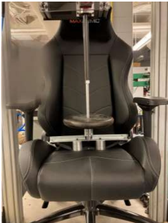
Figure 10. Maxnomic Dominator with the 40-mm LCI 300 seconds after nominal load was applied
