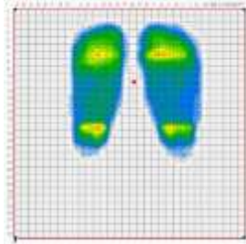
Figure 48. Sample Pressure Mapping output for the All33 Backstrong 60 seconds after load application
