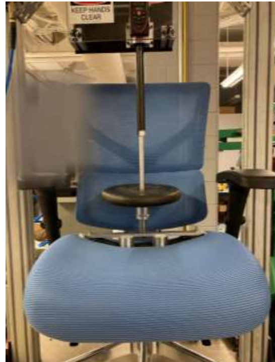
Figure 19. X Chair X3 with the 25-mm LCI 300 seconds after nominal load was applied
