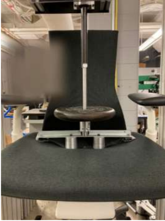
Figure 12. Herman Miller Embody with the 40-mm LCI 300 seconds after nominal load was applied
