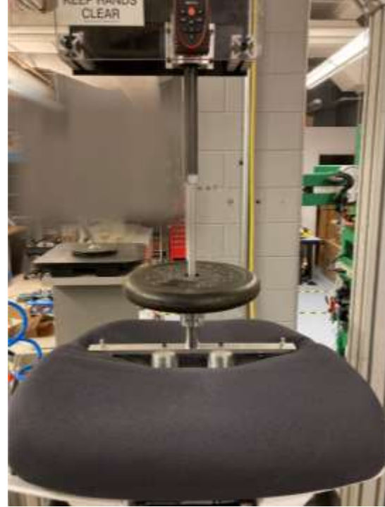
Figure 17. Anthros Chair with the 25-mm LCI 300 seconds after nominal load was applied
