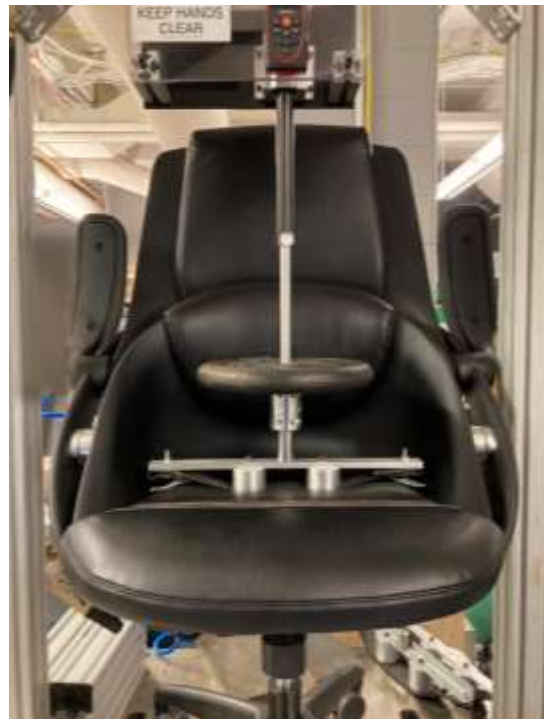
Figure 27. All33 Backstrong with the 25-mm LCI 300 seconds after nominal load was applied
