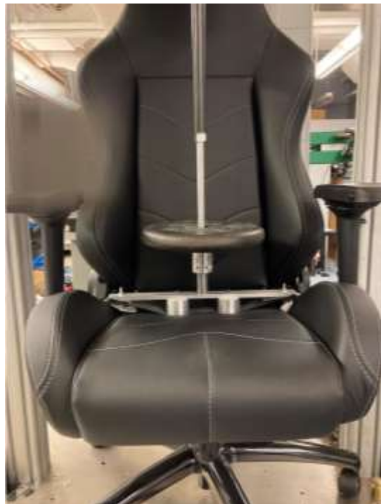
Figure 11. Maxnomic Dominator with the 25-mm LCI 300 seconds after nominal load was applied
