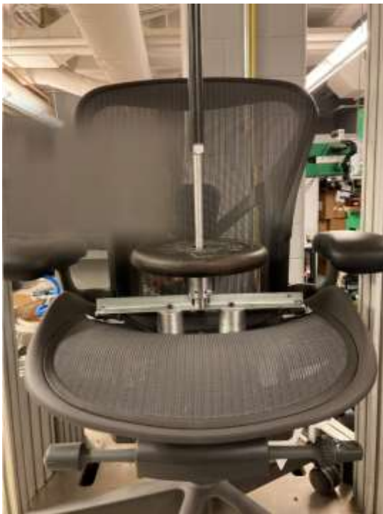
Figure 14. Herman Miller Aeron with the 40-mm LCI 300 seconds after nominal load was applied
