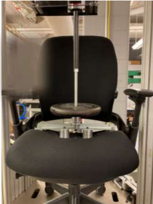
Figure 24. Steelcase Leap with the 40-mm LCI 300 seconds after nominal load was applied
