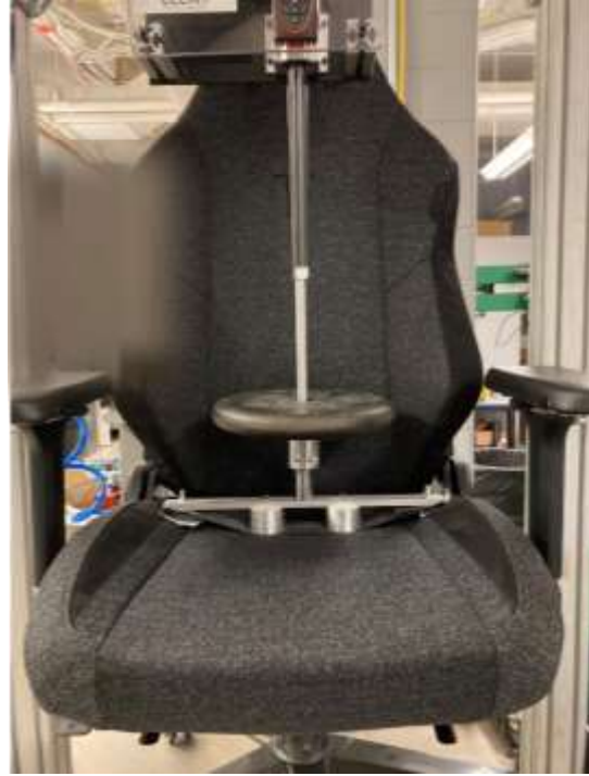
Figure 9. Secret Lab Titan with the 25-mm LCI 300 seconds after nominal load was applied
