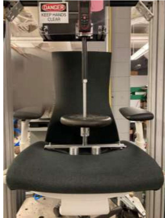
Figure 13. Herman Miller Embody with the 25-mm LCI 300 seconds after nominal load was applied
