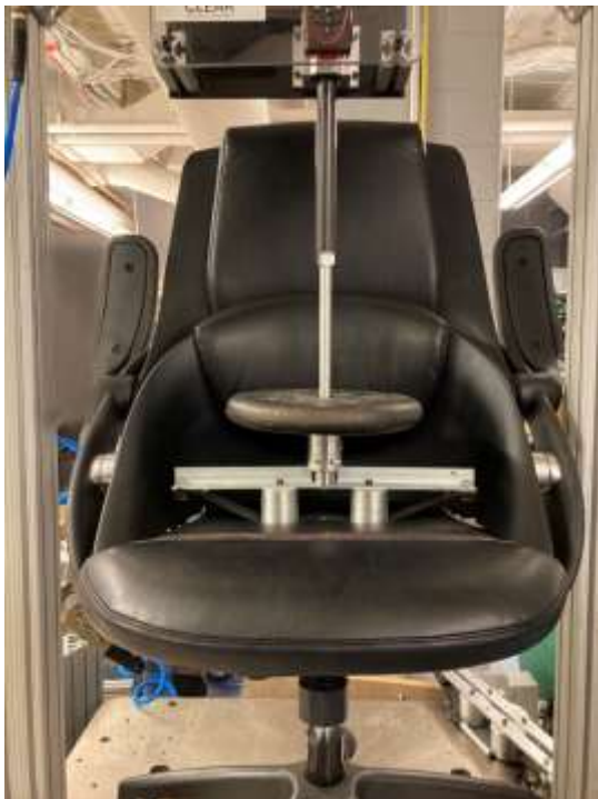
Figure 26. All33 Backstrong with the 40-mm LCI 300 seconds after nominal load was applied.
