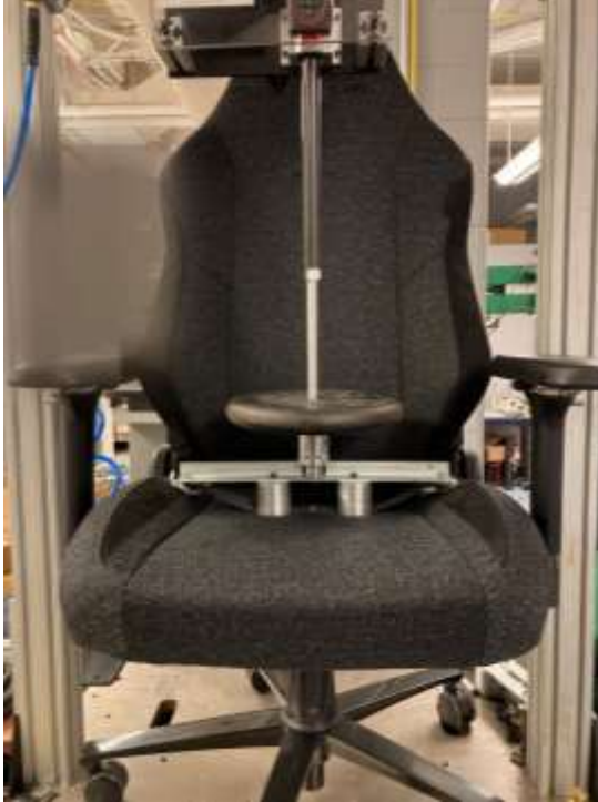
Figure 8. Secret Lab Titan with the 40-mm LCI 300 seconds after nominal load was applied
