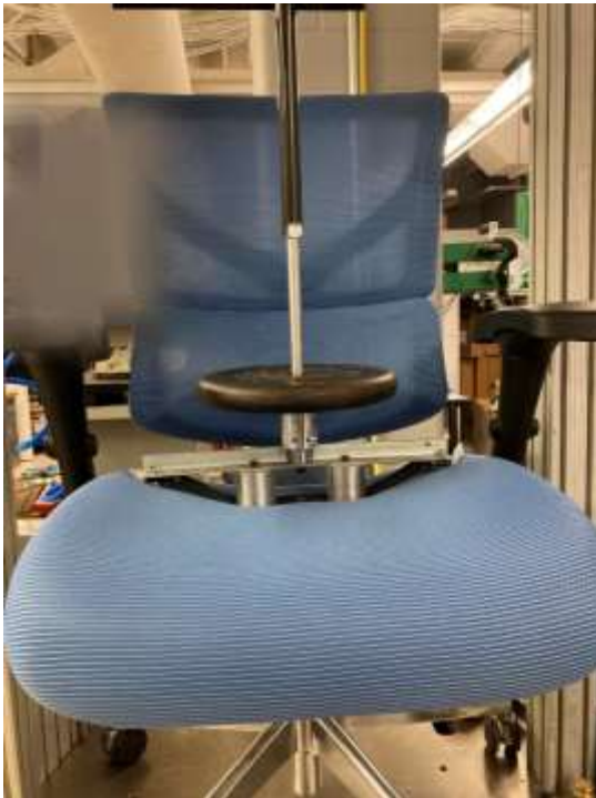
Figure 18. X Chair X3 with the 40-mm LCI 300 seconds after nominal load was applied
