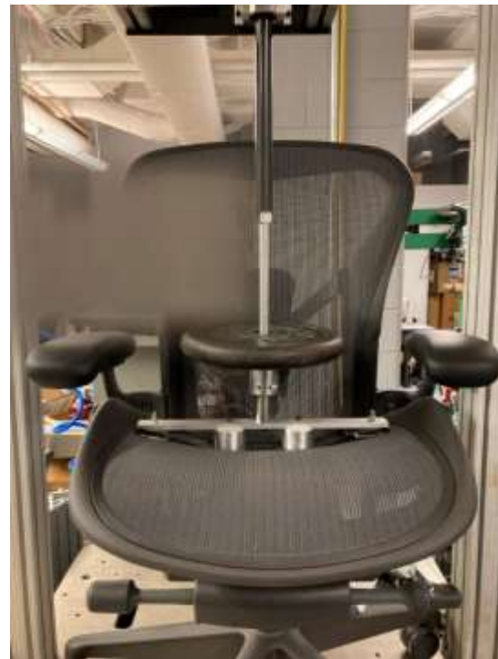
Figure 15. Herman Miller Aeron with the 25-mm LCI 300 seconds after nominal load was applied
